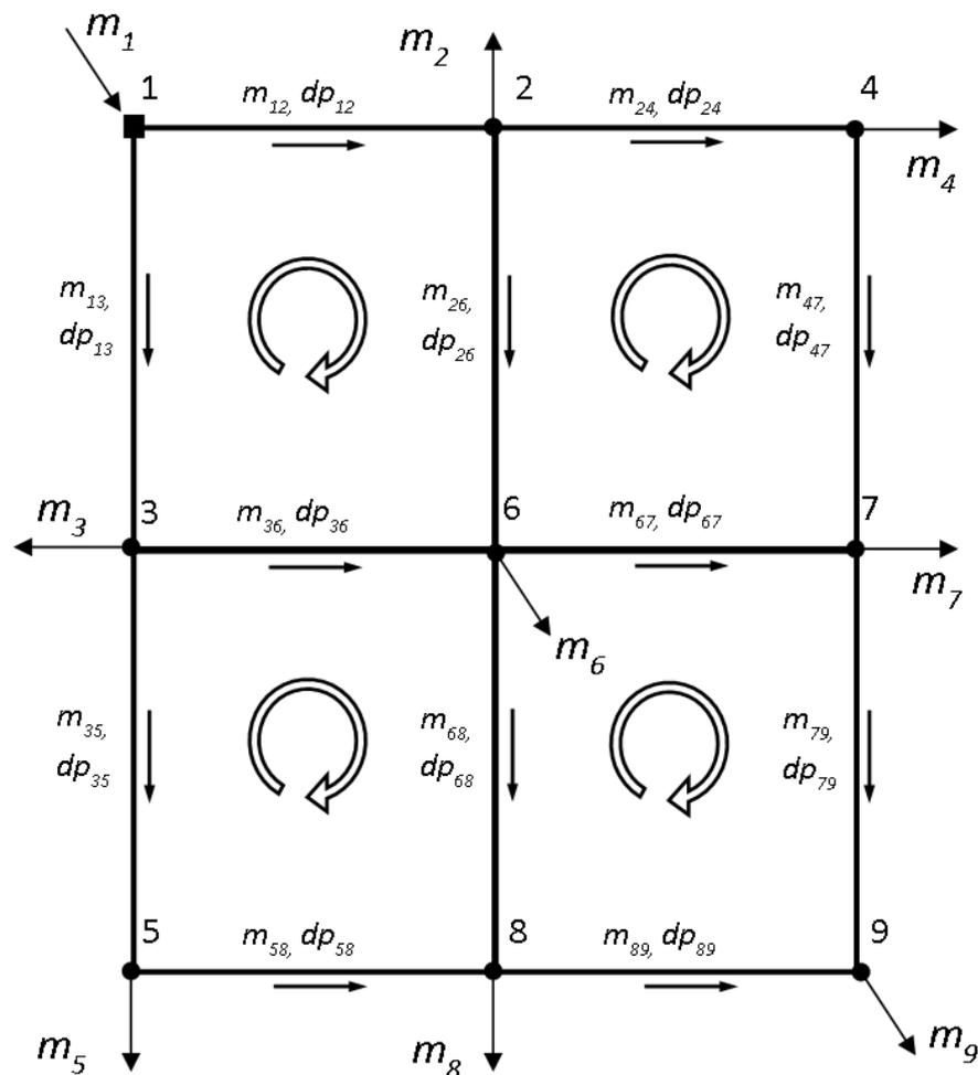
Figure 2. Pipeline schematic to be evaluated
